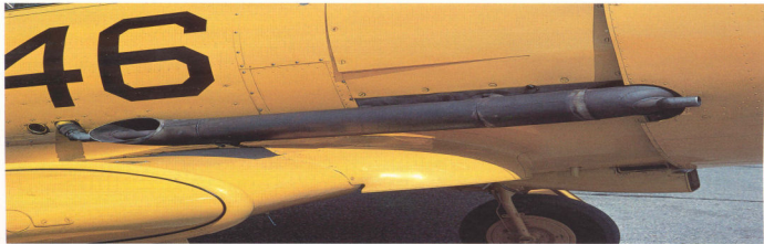
Above Another view of the custom-made exhaust shroud fitted to Canadian Harvards. An effective system which worked exceptionally well, the Pratt & Whitney 'heater' made the Harvard's cockpit the ideal spot to be in on a cold winter's morning
