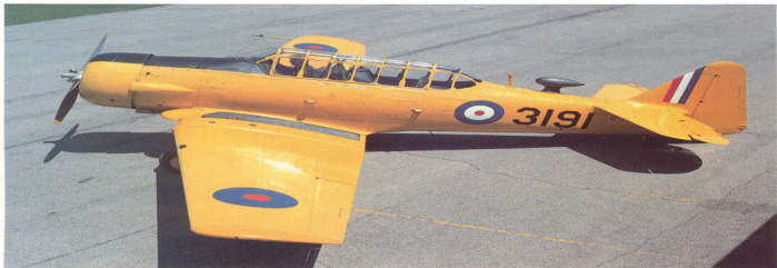
The Harvard II was basically an 'anglicized' AT-6C, its heavily framed canopy contrasting markedly with the later Mk IV. This particular Harvard IIB wears the appropriate wartime scheme of overall gloss yellow, with period roundels and fin flash
